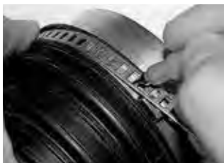
Step 2 Determine the clamp length.
